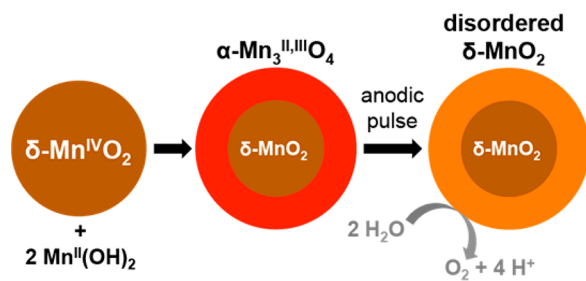
Figure 18. Schematic for the structure of nanosized MnOx domains during activation. First, birnessite ( \delta\text{-MnO}_2 , from constant potential deposition) undergoes surface comproportionation with \text{Mn}^{\text{II}}(\text{OH})_2 , formed by cathodization. The resulting hausmannite ( \alpha\text{-Mn}_3^{\text{II,III}}(\text{OH})_4 ) then converts to disordered birnessite upon anodic conditioning (from either voltage cycling protocols or during oxygen evolution). This disordered birnessite layer is more active toward OER than the original birnessite phase.
